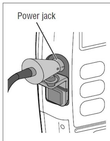
**CAUTION:** Failure to push the connector all the way forward may result in an intermittent connection, and the connector may dislodge, causing a loss of power.
